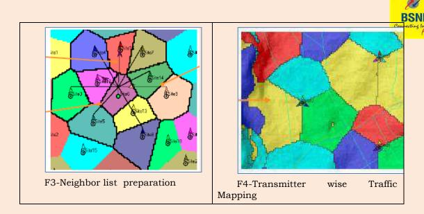
**Figure 1:** This type of mapping is helpful in avoiding co-channel and adjacent channel interference situations. The availability of this data with O&M teams and OMCRs is useful in frequency planning during any type of network modification or new site addition work. Other benefits include subscriber complaint attendance and marketing purposes.
